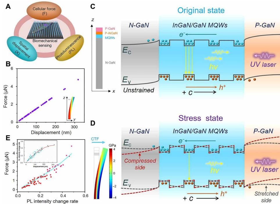
**Fig. 4. Mechanism of CTF measurement based on the PLNA array.** (A) Three core parameters involved in CTF monitoring. (B) Relationship of cell force and displacement of the PLNA. (C and D) Band diagram for understanding the PL change of the PLNA under cell traction. (E) Experimental (red dot) and fitting (violet line) results of the cell force upon the photoluminescence intensity change rate.
